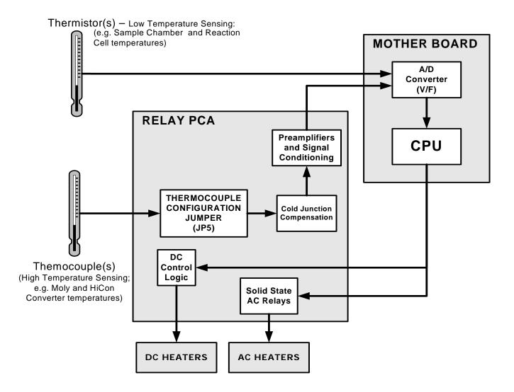
Figure 2-7: Heater Control Loop Block Diagram.
